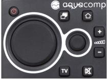
Three keys of the aquaremote select the mode of operation: "VISION" mode is selected by pressing the "a" key, the "a" key selects "Computer" mode and "Media" mode can be selected by pressing the "TV" key. The currently selected mode is displayed on the VISION module display for approximately two seconds after switching modes. The circular mouse control pad
