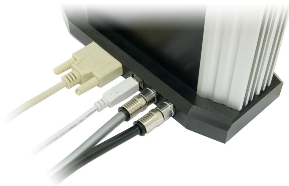
All aquaduct variants have two electrical and two hose connections. The left 15-pin connection serves for the power supply of the aquaduct and always has to be connected with the PC interface circuit board. **Important:** Attach this plug only to the enclosed interface! It is **not** a PC standard connection!
