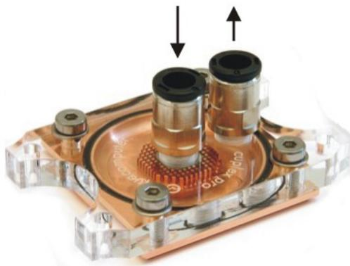
Unlike channel coolers, the microstructure coolers cuplex kryos and cuplex PRO have a predefined flow direction. The coolant must be led in through the central connection directly onto the microstructure, the coolant is then led out through the lateral connection. In order to attain the full performance of the waterblock, correct connection of inlet and outlet is crucial.
