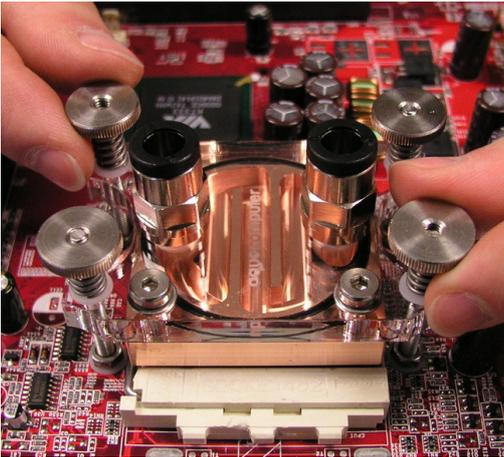
Screw one of the supplied knurled nuts on each screw about 2 turns, so it just grips. For fastening the springs, take turns in fastening two knurled nuts at a time placed opposite of each other diagonally. During this process make sure that the **spring coils do not touch each other**, since this can cause inadmissible high forces to build up. The spring has to
