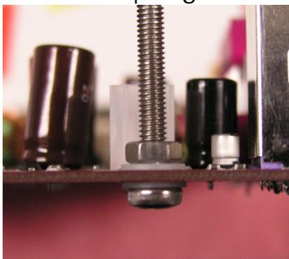
that purpose detach your motherboard from the computer case. In P4- and Xeon-systems the mostly black plastic mounting for air-coolers has to be removed from the motherboard to reveal the necessary drill holes on it. Next slide a plastic washer over one of the supplied stainless steel M4 screws which you then put through the holes adjacent to the socket from below. Slide
