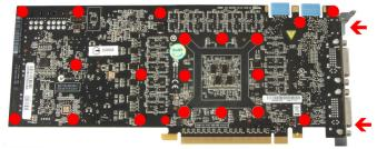
dicated with red dots in the figure. Use extreme caution not to damage any of the highly sensitive components of the graphics card! Disconnect the fan connector while lifting the air cooling unit off the graphics card.
