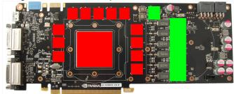
Apply a thin layer of thermal compound to the GPU and the RAM modules. These components are marked red in the figure. The thermal compound must not be electrically conductive! Cut fitting pieces from the thermally conductive pad supplied with the aquagraFX and place them on top of the voltage regulators as indicated by green rectangles.
