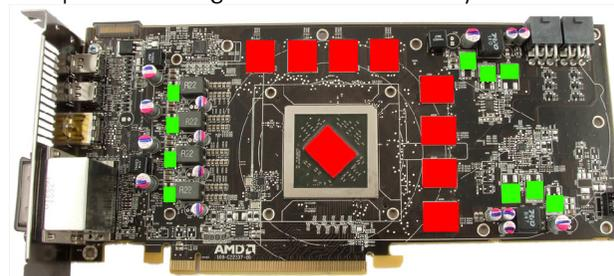
Apply a thin layer of thermal compound to the GPU and the RAM modules (indicated by red marks in the figure). The thermal compound must not be electrically conductive! Cut fitting pieces from the thermal pad supplied with the waterblock and place them on top of the voltage regulators (indicated by green marks in the figure).
