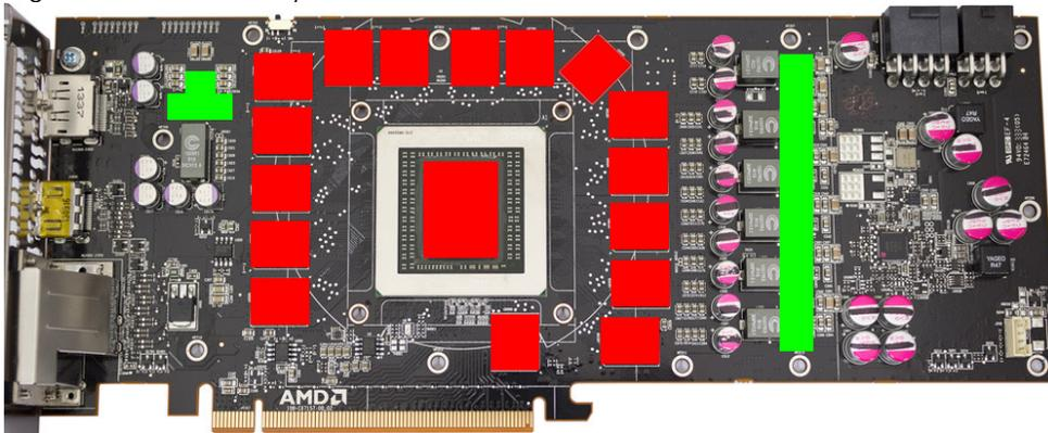
Apply a thin layer of thermal compound to the GPU and the RAM modules. These components are marked red in the figure. The thermal compound must not be electrically conductive! Cut fitting pieces from the thermally conductive pad supplied with the kryographics and place them on top of the voltage regulators as indicated by green rectangles.
