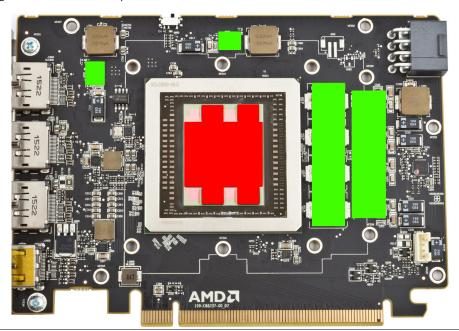
Apply a thin layer of thermal compound to the GPU with HBM modules. These areas are marked red in the figure. The thermal compound must not be electrically conductive! Cut fitting pieces from the thermally conductive pads supplied with the kryographics and place them on top of the components as indicated by green rectangles.
