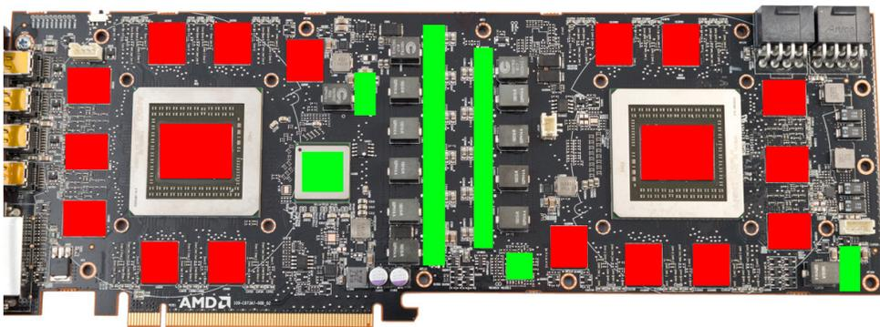
Apply a thin layer of thermal compound to the GPUs and the RAM modules. These components are marked red in the figure. The thermal compound must not be electrically conductive! Cut fitting pieces from the thermally conductive pad supplied with the kryographics and place them on top of the voltage regulators and PCIe switch as indicated by green rectangles.
