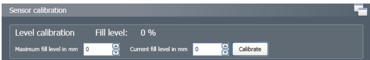
Before the sensor can produce accurate readings, it needs to be calibrated. To do so, use a folding rule or measuring tape to determine current fill level and maximum fill level of your reservoir and enter the values into the corresponding boxes of the software. After confirming these values by clicking "Calibrate", the software will generate the calibration data.
